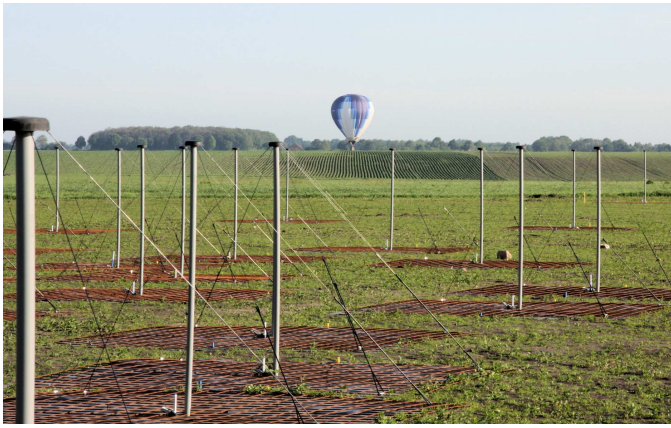
Fig. 1. LOFAR low band antenna sparse pseudo-random array.
