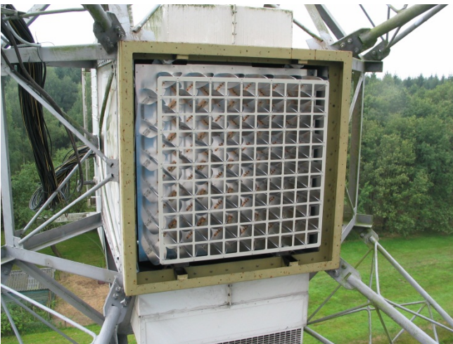
Figure 5. APERTIF PAF prototype system mounted in the prime focus of one of the WSRT dishes as seen from the reflector.
