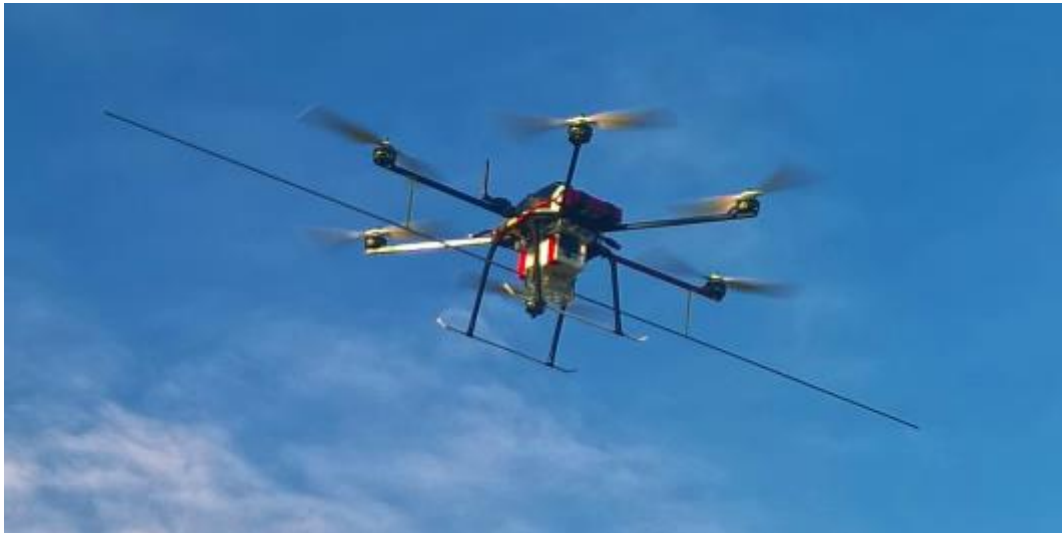
Figure 2. The flying artificial test source consisting in the UAV equipped with the RF transmitter and the 2-m long dipole antenna.
