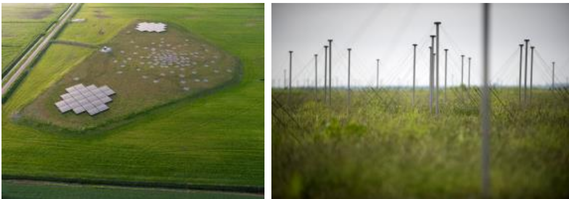
Figure 1. Aerial photograph of a Dutch LOFAR station made by Top-Foto (left) and a photo of the LBA array taken by Hans Hordijk (right).
