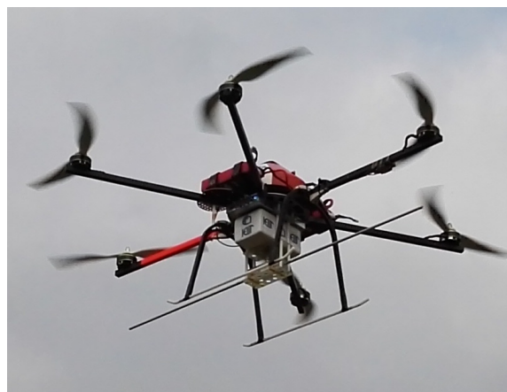
Figure 1. The hexacopter carrying the RF transmitter (white box) and the dipole.
