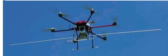
Figure 1: UAV-based flying test source. The payload consists of a GNSS receiver, an RF generator and a dipole antenna.
