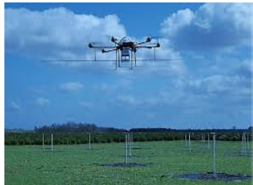
Fig. 1. UAV-based system flying during a measurements campaign on a LOFAR LBA station located in The Netherlands.
